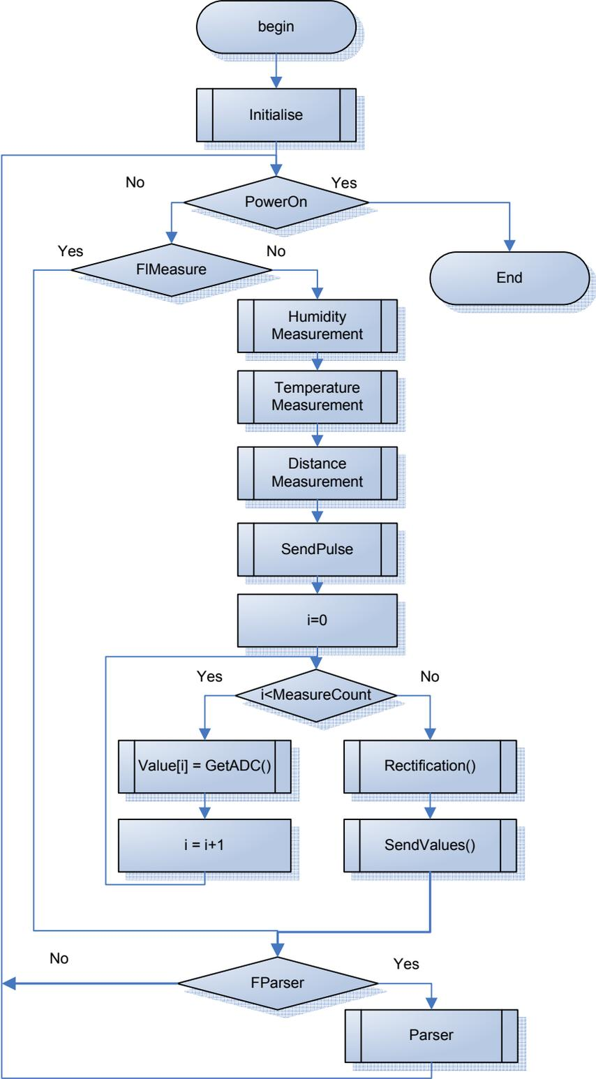
Figure 3: Algorithm of operation about receiver-transmitter module
