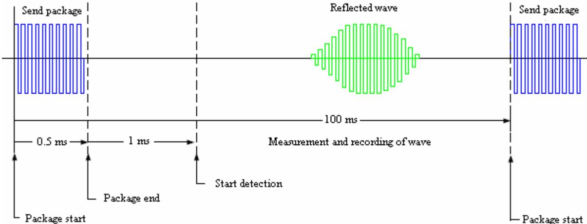
Figure 2: Scheme showing the operation principle of blocks: receiver and transmitter
