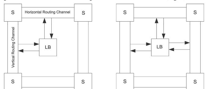
Fig. 3. Input/outputs pad of the logic group
