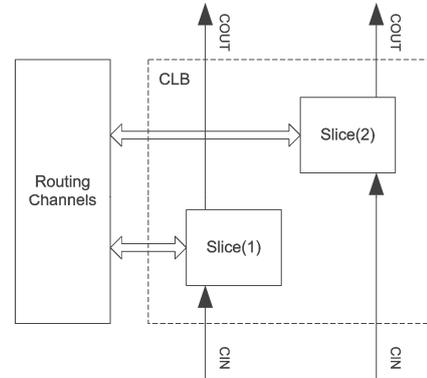
Fig. 5. Arrangement of Slices within the CLB
