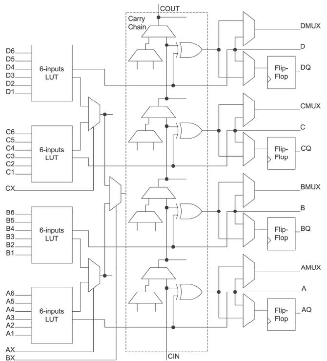
Fig. 6. Structure of the slice element within Virtex-5
