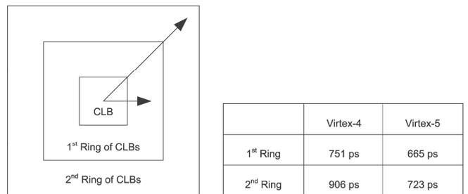
Fig. 9. Routing Delay Comparison for Virtex-4 and Virtex-5
