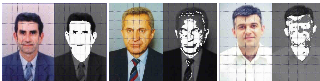
Fig. 7. Adaptive skin detection – disturbed white balance (source http://www.tugab.bg )
