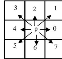
Fig. 2 Direction vectors in chain code
